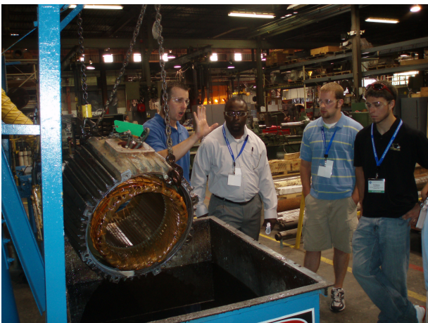
A reconditioned stator that has been coated.
